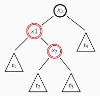
BST property:  $t_1 < x_1 < t_2 < x_2 < t_3 < x_3 < t_4$
