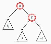
First we recursively fuse the *middle subtrees*:  $s = fuse t_4 t_5$ If s has a black top node, we put it under y
