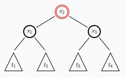
BST property:  $t_1 < x_1 < t_2 < x_2 < t_3 < x_3 < t_4$ If the consecutive red nodes are in the right child rotate symmetrically in the other direction
