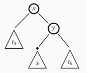
Again we recursively fuse the *middle subtrees*:  $s = fuse t_4 t_5$ If s has a black top node, we put it under y
